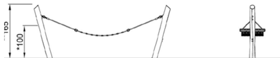
Incidental play - 2no hammocks in the cherry orchard Age group: 3+ Play capacity: 2 users Materials: timber, PES ropes, stainless steel brackets
